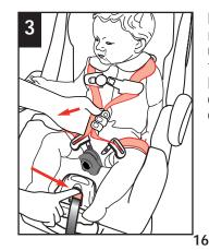
Push down on harness release button while pulling up on harness straps above the latch plates to loosen. Place harness over sides of child restraint. Remove child.
